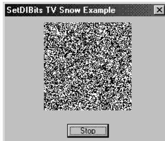
Figure 12-20: The DDB image was set from bits stored in a DIB
